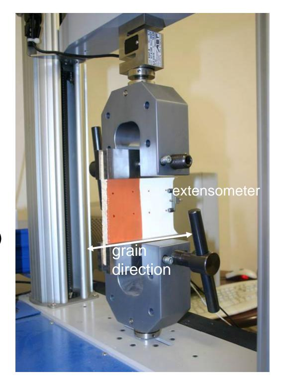
Direct tracing of damage development at the micro-level using ESPI (Electronic Speckle Pattern Interferometry):
