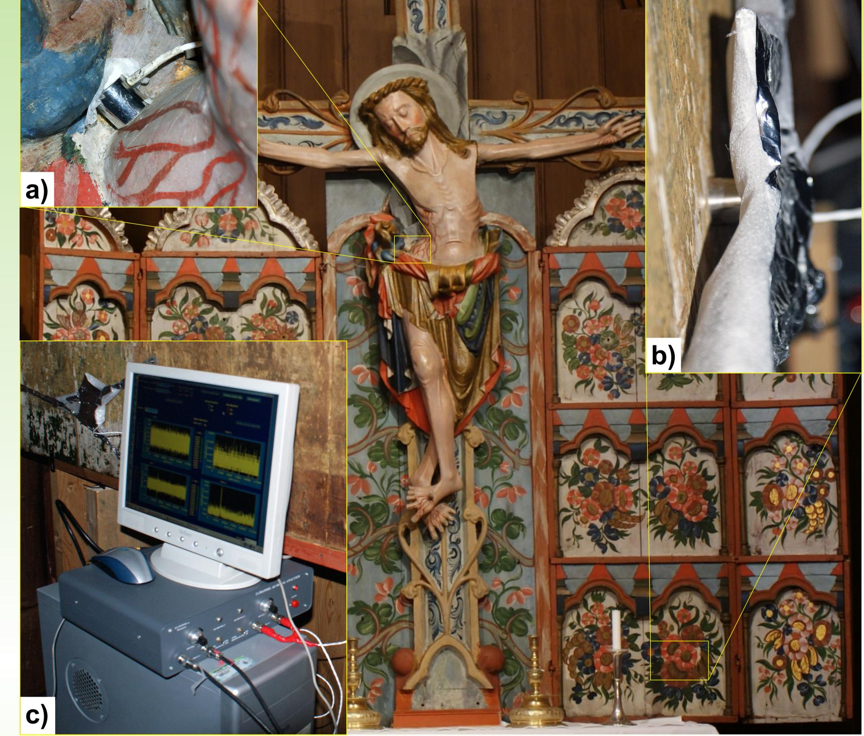
Acoustic emission (AE) is defined as energy released due to micro-fracturing of materials under load. The energy passes as ultrasound and sound waves, and is detected at the surface using a piezoelectric sensor which converts the surface vibration to an electric signal. The AE monitoring has become an important non-destructive tool to gain insight into the evolution of damage in materials.
