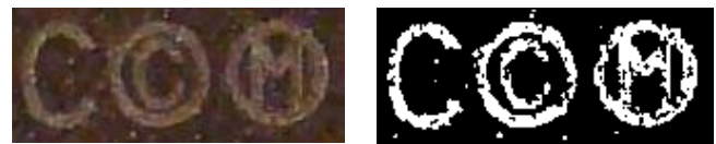
Fig.3 Original pictures (top and bottom left) and enhanced (bottom right) with binarisation (128/256)
