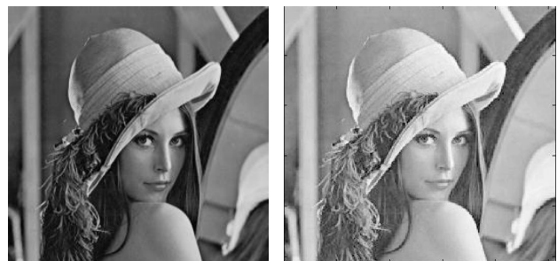
Fig 1. Original image lena.tif and its brighter copy Using division, multiplication, subtraction, roots or powers, one can increase or decrease value of pixels, making picture lighter or darker. Often, result of computation has to be normalised to be within uint8 limits ( 0..255 ). Some results are given on figure 1.
