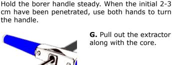
come out of the tip. If you do not have a borer starter available, guide the penetration with one of your hands and gently push and turn clockwise with the other hand at the centre of the borer handle.
