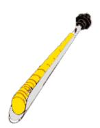
H. The core is ready to be examined. Gently unscrew the borer auger from the tree.
