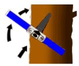
The borer is now ready for use.When screwing the borer into the tree, consider the following: Do not use force starting when the penetration. It may cause damage to your borer and small chips may
