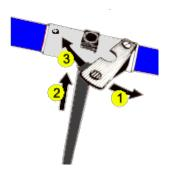
C. Turn the lock and insert the auger (bit) in the handle. Then gently turn back the lock until the auger is secured into the handle.
