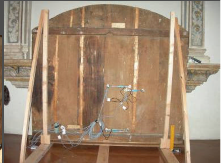
(3 DKs mounted on the Tryptich)
