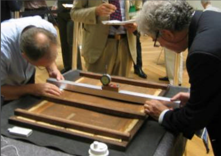
Manual measurement of deflection
