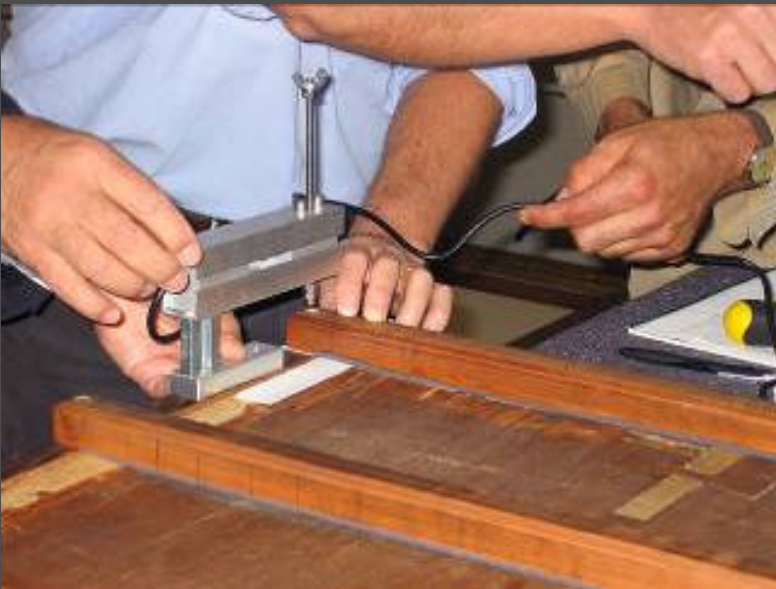
Manual measurement of deflection
