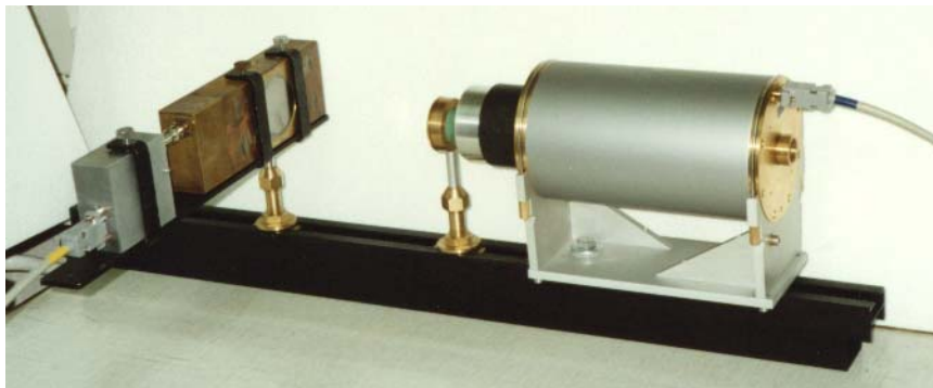
Fig. 1. Basic set-up of the spectrometer with the proportional detector.
