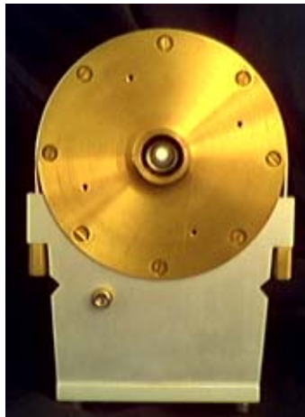
Fig. 6. Front end of the transducer. See, the hollow central tube.
